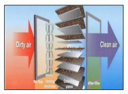
Fig. 1 Working Principle of Electrostatic Precipitator Construction
