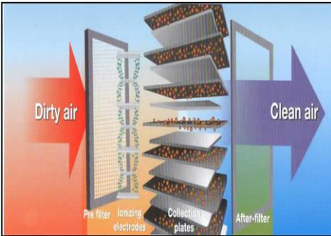
Fig. 1 Working Principle of Electrostatic Precipitator
