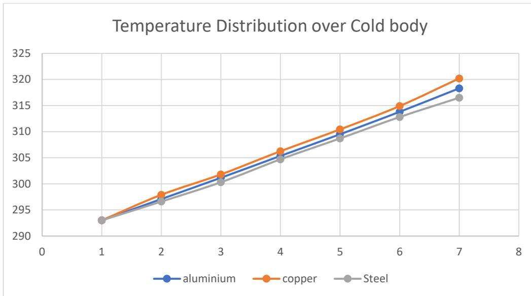
The **Cold fluid's temperature Increases steadily** along the length of the shell for all materials, influenced by their thermal conductivity and heat transfer performance.
