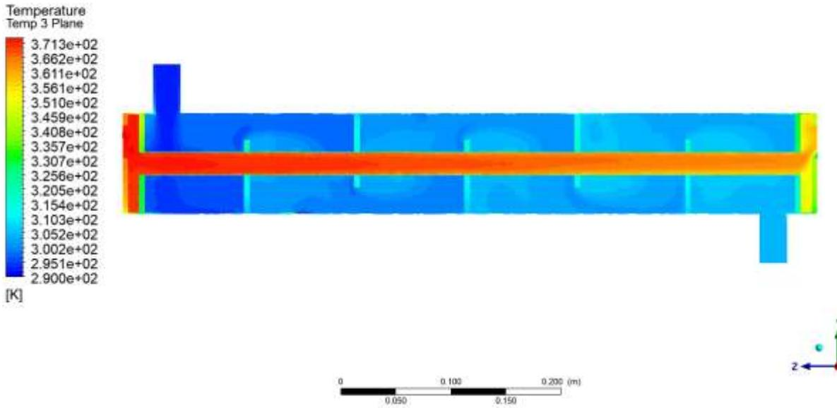
Figure 13 Temperature distribution over Plane
