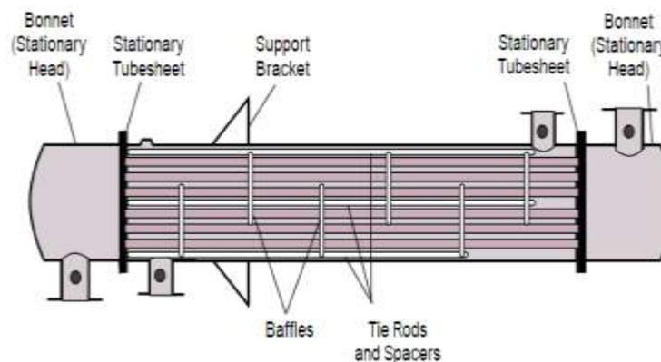
Figure 1: shell and tube heat exchangers (Mukherjee, 1998) [2]
