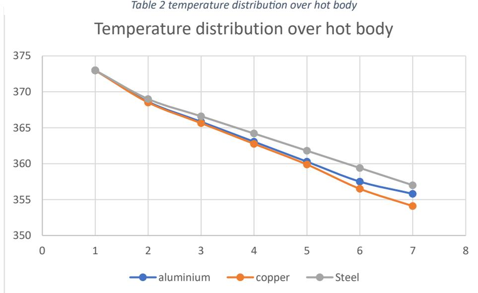
The hot fluid's temperature decreases steadily along the length of the shell for all materials, influenced by their thermal conductivity and heat transfer performance.
