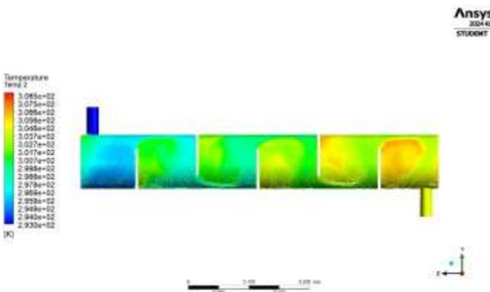
Figure 11 temperature Contour over shell
