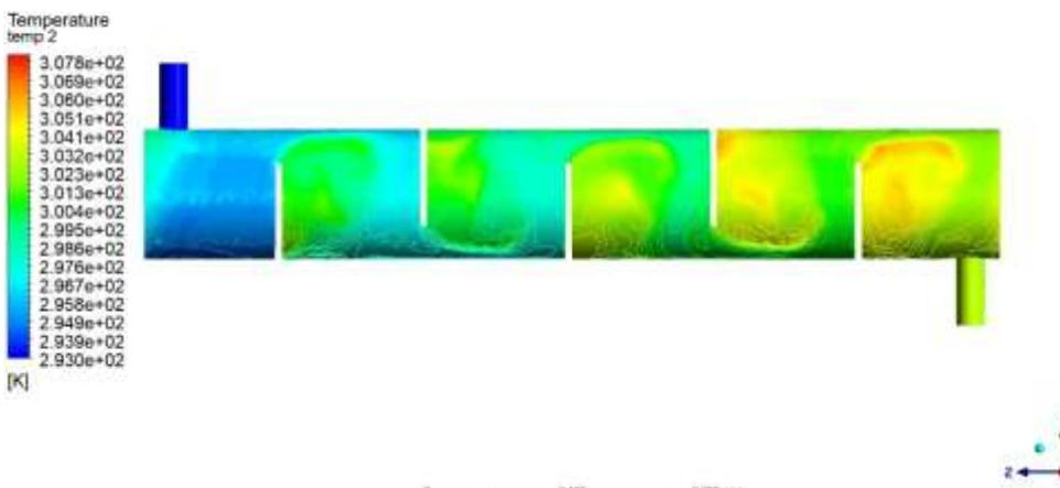
Figure 14 temperature Contour over shell and tube heat exchanger
