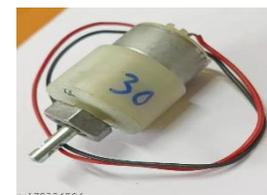
Fig.4: DC GEAR MOTOR
