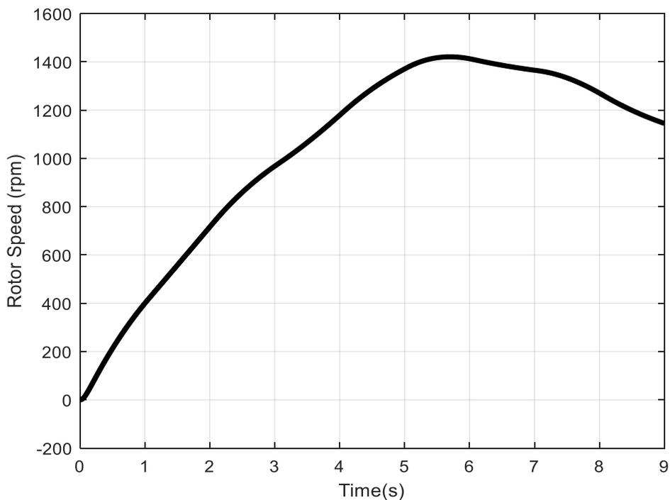
**Figure 9: Rotor speed of DC motor for HPSOGSA algorithm**
