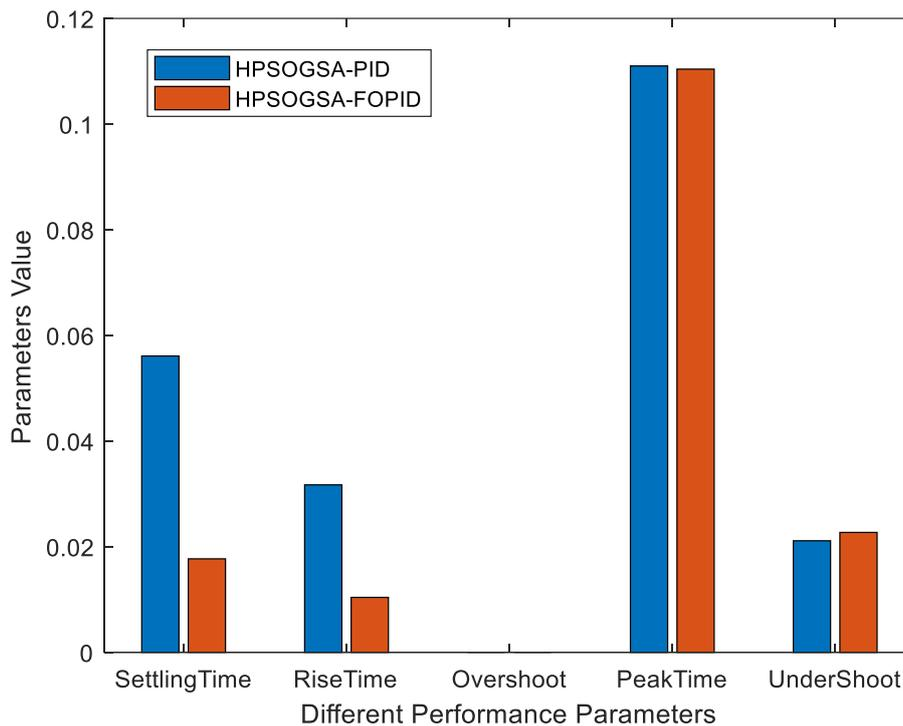
**Figure 10: Comparison of fitness parameters for HPSOGSA-PID and HPSOGSA-FOPID models.**
