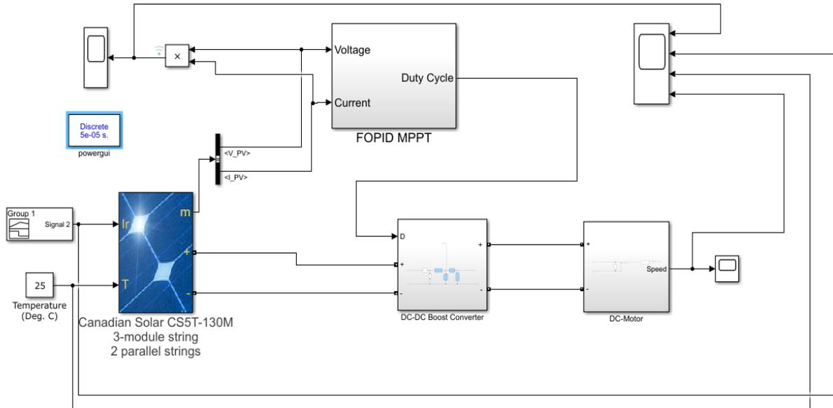
**Figure 1: Schematic of SPV based Smart Battery Charging System**
