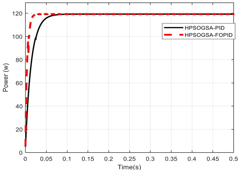
**Figure 6: Comparison of penal power versus time for HPSOGSA algorithm using PID & FOPID controllers**
