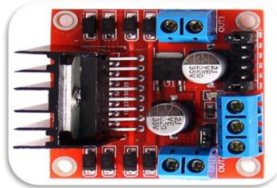
Fig.5 L298n motor driver module
