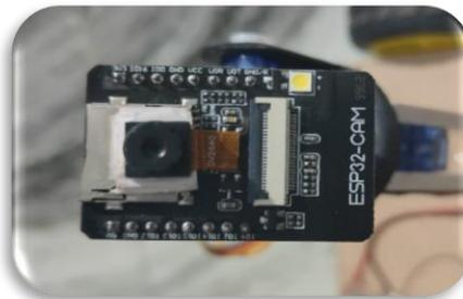
Fig.9 Esp-32 camera module
