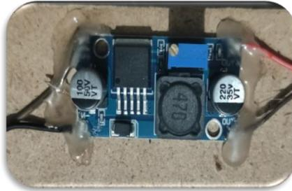
Fig.8 Lm2596 dc step-down buck converter
