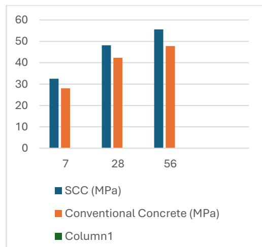
SCC exhibited higher compressive strength at all ages due to improved compaction and continuous pozzolanic reactions.
