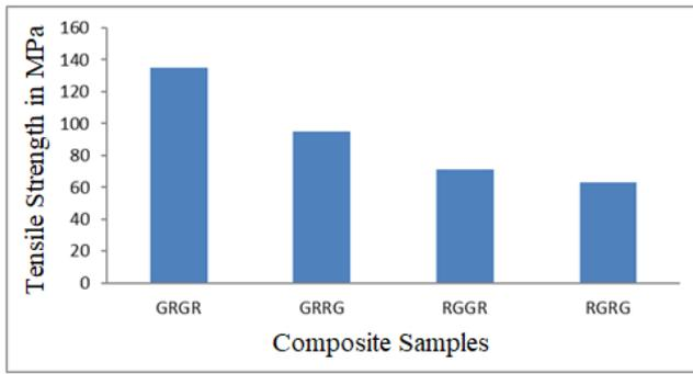
**Fig - 3:** Composite tensile strength of Fiber Glass with Rubber layer
