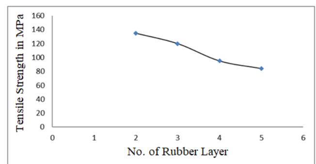
**Fig - 2:** Composite tensile strength with Rubber layer
