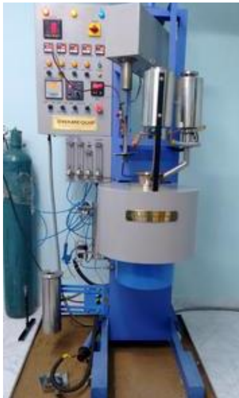
Fig -1: Stir Casting Setup
