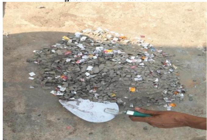
Fig: Mixing of Concrete with medical strips as per mix
