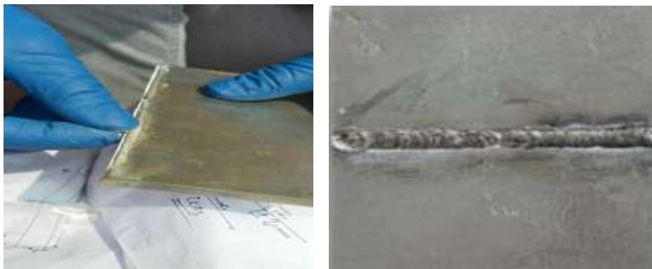
Figure.8 (a) Filling of cerium oxide powder in the grooves (b) Weldment specimen
