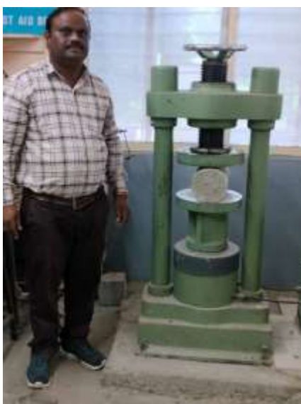
Fig. 3.3 : Split Tensile Strength Testing
