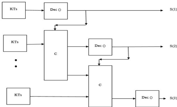
Fig. 2. The conceptual model for successive signal detection
