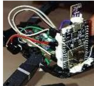
Fig 3: Interfacing of Buzzer with NodeMCU
