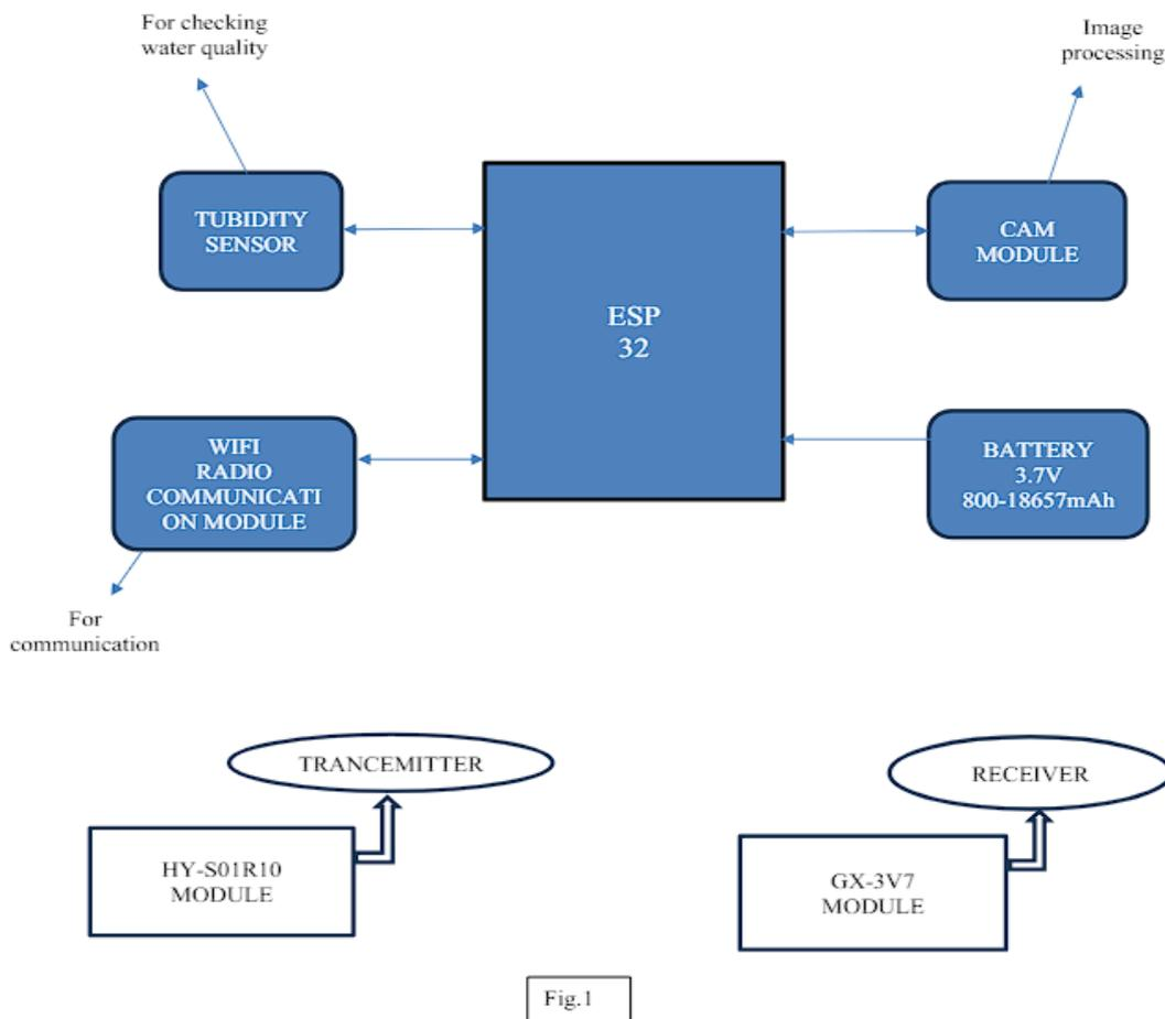
Figure 3.1: Block diagram
