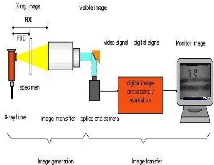
Fig-4 Radioscopic inspection system
