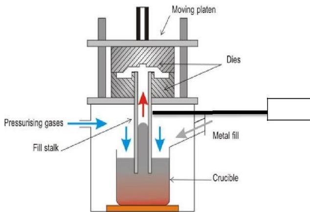
Fig-3 Low pressure die casting
