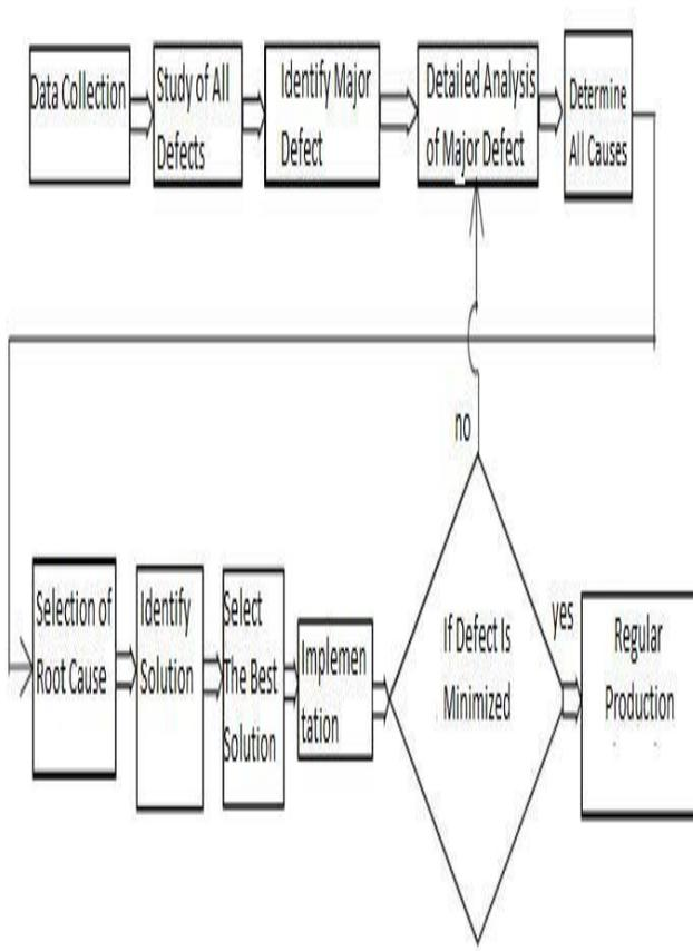
Fig-5 Defect diagnostic approach
