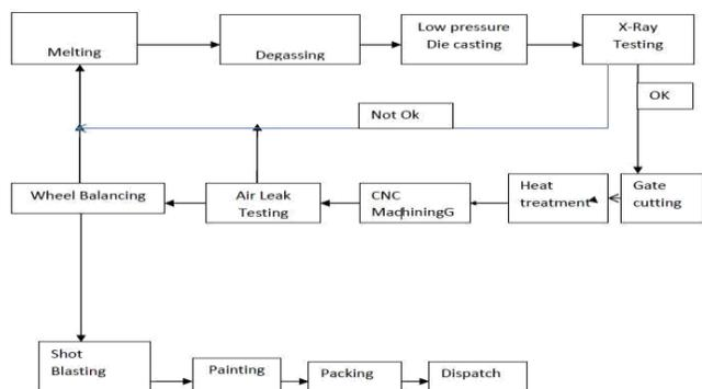
Fig-1 Process flow diagram for manufacturing of Al alloy wheel
