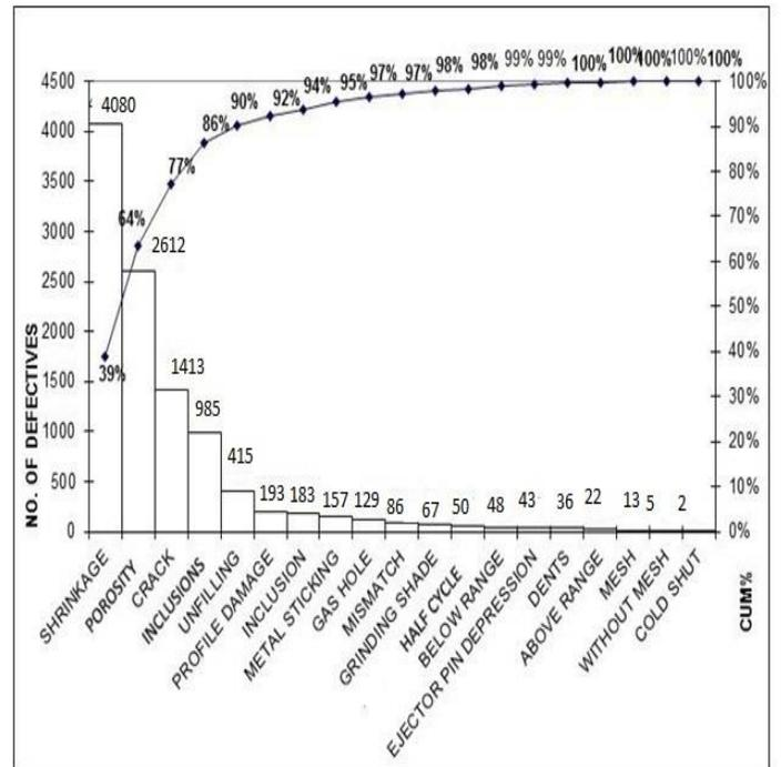
Fig-6 Pareto chart of rejections of Al alloy wheels for one year
