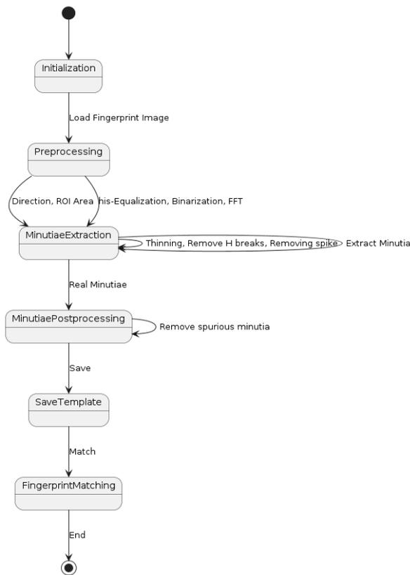
Figure 1. Purposed flowchart diagram
