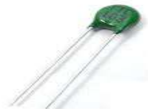
Fig no 9. Temperature sensor (NTC)
