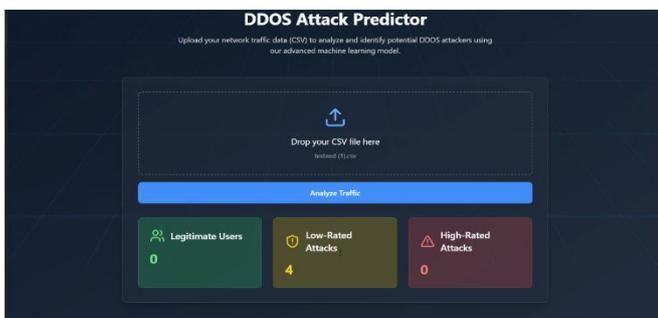
The Dashboard Module provides a user-friendly interface for displaying detection results. It showcases the number of legitimate users, Low-Rate attacks, and High-Rate attacks in an interactive format. Visual elements, such as graphs and tables, ensure clear representation, helping users quickly assess network activity.
