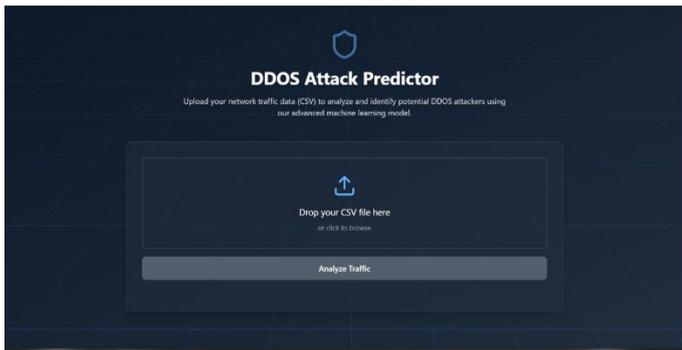
The Data Upload Module allows users to upload network traffic data for analysis. A structured interface enables users to submit PCAP or CSV files, which are validated to prevent corrupt or malformed data. Real-time file processing mechanisms extract relevant features such as packet rate, request frequency, and IP distribution, ensuring that uploaded data is efficiently processed for attack classification.
