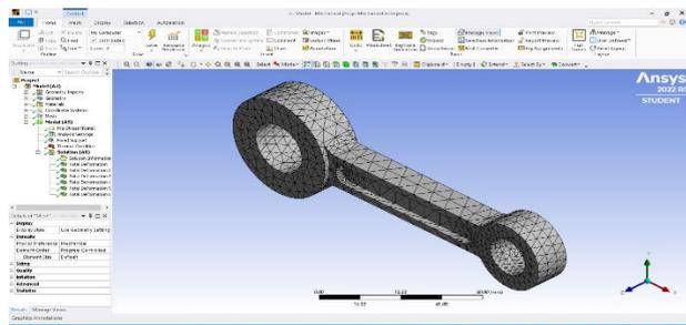
**Step-6:-** Analysis settings are set for modal analysis of six nodes and the required solutions are added.
