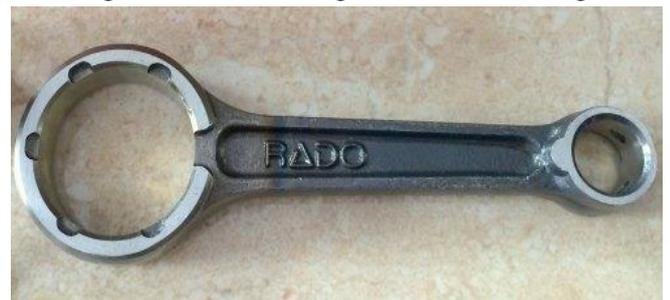
Fig.2 Two-Wheeler Connecting Rod
