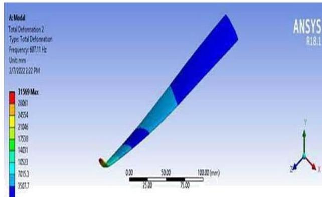
Fig.5 Nitrile 60 shore A rubber treated blade for Mode 2: 607.11 Hz
