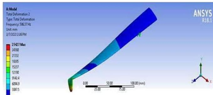
Fig.7 Nitrile 80 shore A rubber treated blade for Mode 2: 586.37 Hz
