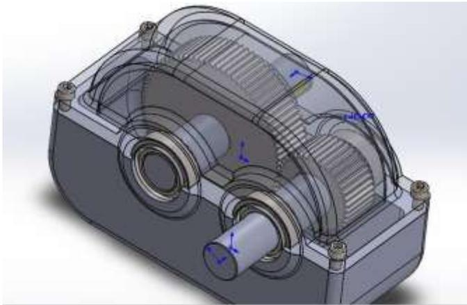
**Fig -1:** Assembly of Driver Transmission
