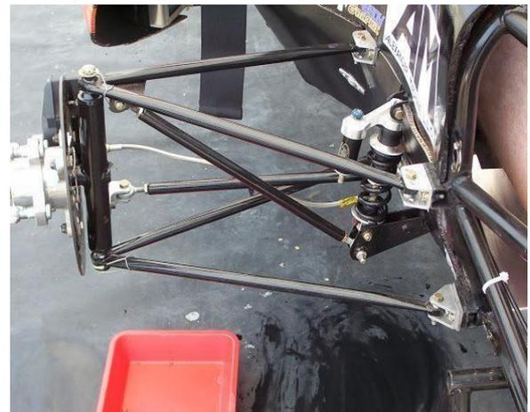
**Fig.1. 8.** Double-wishbone pull rod suspension
