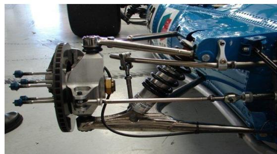
**Fig.1.5.** Double-wishbone suspension
