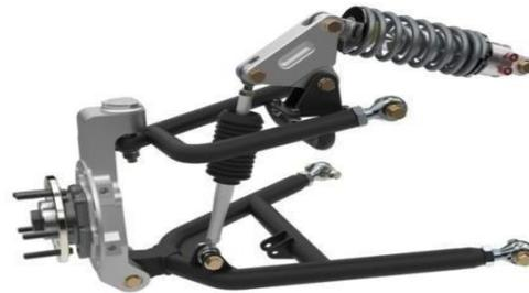
**Fig 1.7.** Double-wishbone pushrod suspension
