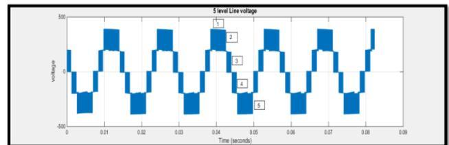
5.5 Five Level multilevel inverter with induction motor load
