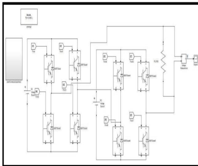
4.6 Five-level multilevel inverter with induction motor load
