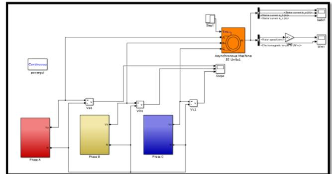
4.7 T Type multilevel inverter with induction motor load
