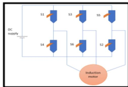
The inverter is a device that converts DC supply to AC supply. The inverter operates in 180-degree and 120-degree conduction modes. Three-phase induction motor work on AC supply for that required convert DC boost voltage to AC supply. The induction motor operates on 180-degree conduction mode inverter.
