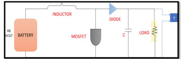
As shown in figure here taking a 48-volt battery that needs to boost voltage at 400- volt as per induction motor required input. for that here take 0.88 duty ratio of MOSFET. During Ton time inductor stores the energy. At that time diode reverse bias. During Toff time inductor energy and battery energy are both added and given to the resistive load at that time diode forward bias. Here capacitor work as a filter that is used to eliminate distortion.
