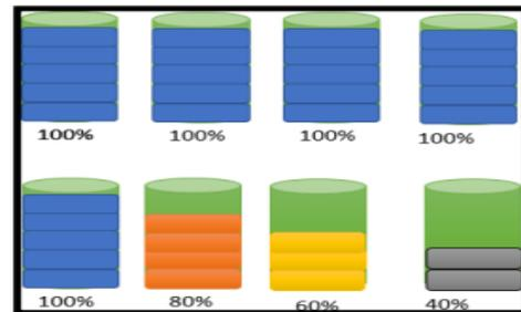
Here as shown in fig .there are 2 conditions first is the ideal condition and the second is practical. In Ideal conditions, all batteries have the same states of charge and voltage levels but it is not possible practically. In practically all batteries different states of charge and voltage level so, to make all batteries same level and provide working we use the cell balancing process
