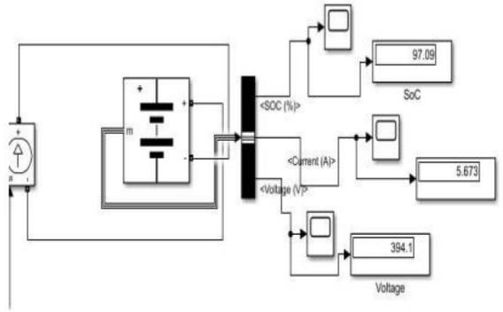
**Fig. 11. SoC of battery with actual set parameters**
