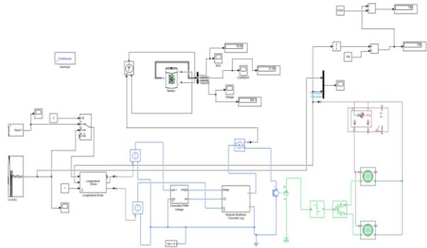
**Fig. 3. Simulation of electric vehicle with H-Bridge**
