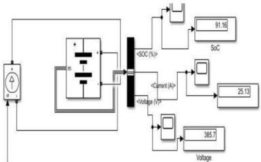
**Fig. 12. SoC of battery with newly set parameters**
