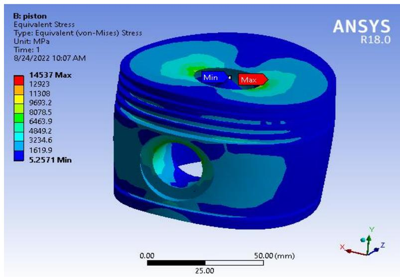
Figure 6 Equivalent Stress
