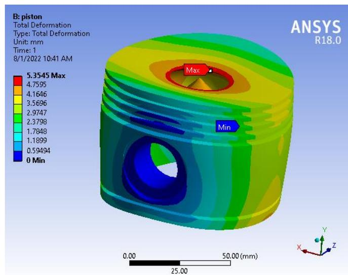
*Figure 2 Total Deformation*
