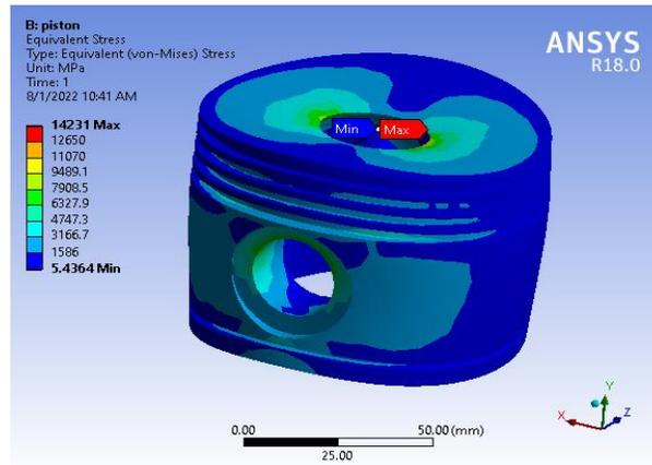
Figure 3 Equivalent Stress
