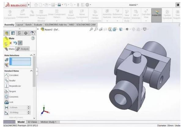
Fig-3: Model of Universal Coupling
