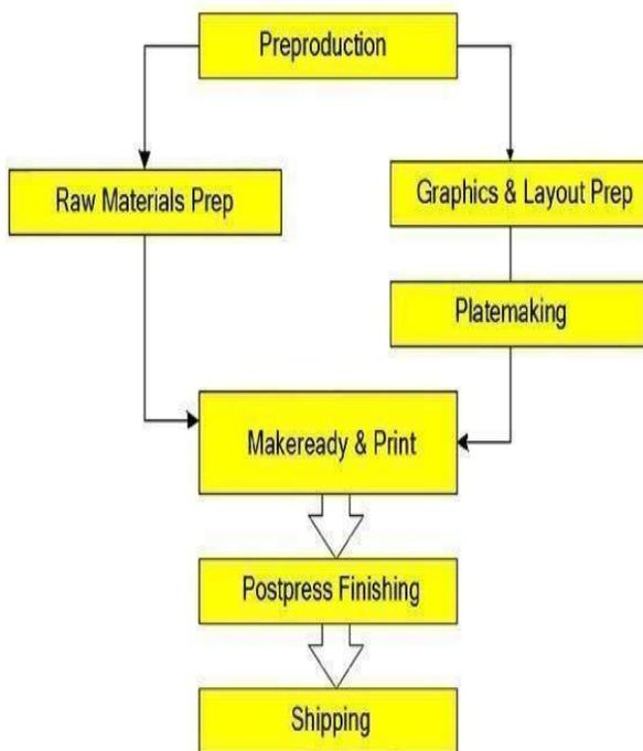
Fig-2: Printing process flow chart
