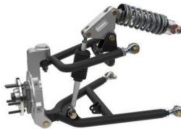
Figure 8: Double-wishbone pushrod suspension
