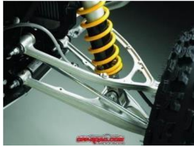
Figure 5: Double wishbone setup
