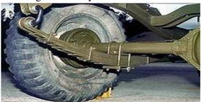
A leaf spring is a simple form of spring commonly used for the suspensionin wheeled vehicles. Originally called a laminated or carriage spring, and sometime referred to as a semi elliptical spring or chart spring, it is one of the oldest forms of springing, dating back to medieval times.
