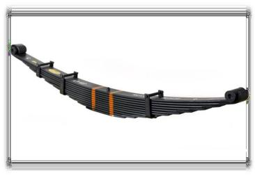
Additional suspension components, such as trailing arms, would usually be neededfor this design, but not for "semi-elliptical" leaf springs as used in the Hotchkiss drive.
