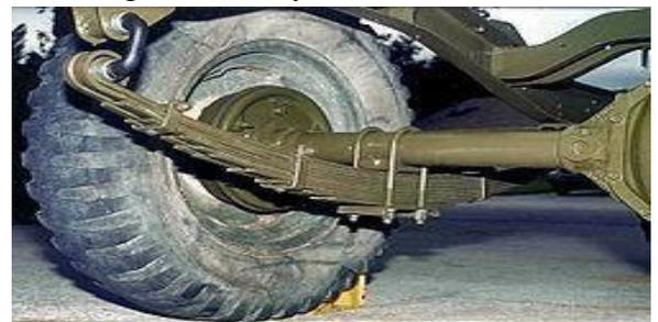
A leaf spring is a simple form of spring commonly used for the suspension in wheeled vehicles. Originally called a laminated or carriage spring, and sometime referred to as a semi elliptical spring or cart spring, it is one of the oldest forms of springing, dating back to medieval times.
