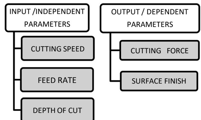
Figure 1: Parameters of Aluminum 6061 Alloy
