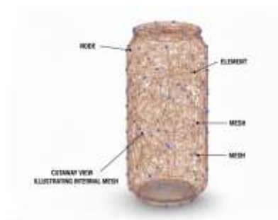
Fig 1: A beverage bottle showing mesh structure for FEA modeling
