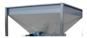
The hoppers are used to feed the conveyor systems with the products to be dosed, Hoppers a hopper is used to hold bulk materials before they are transferred into a conveying system, bag, or container for use or for distribution. The hopper is designed to temporarily store bulk materials until they need to be emptied out into something else through a discharge port on the bottom.
