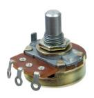
A potentiometer is a type of position sensor. They are used to measure displacement in any direction. In Linear Potentiometers the track is straight and in Rotary the track is circular. The wiper moves along the track to measure the displacement through proportionally dividing the input voltage
