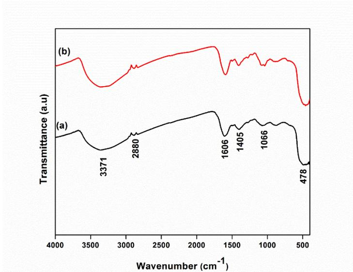
Fig. 3. FTIR spectra of ZnO (a) 1h (b) 3h
