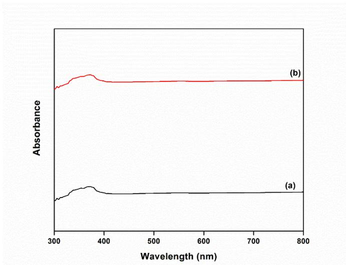
Fig. 4. UV-Vis Absorption Spectra of ZnO (a) 1h (b) 3h
