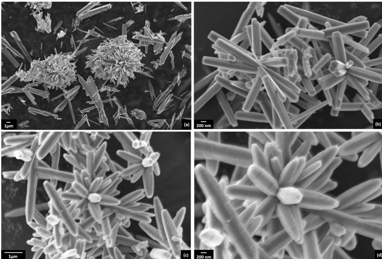
Fig. 5. FESEM images of ZnO (a,b) 1h and (c,d) 3h
