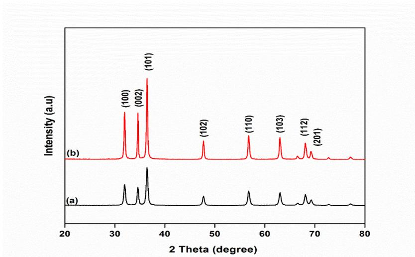
Fig. 2. XRD pattern of ZnO obtained by varying the reaction period of (a) 1h and (b) 3h
