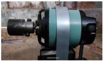
B. **Rotary hacksaw** The rotary hack saw is directly connected to the end of the motor shaft. As it directly connected to the motor shaft the speed of the rotary hacksaw equal to the motor speed.
