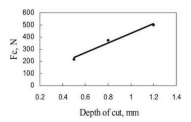
2. cutting forces and depth of cut are directly related If the depth of cut increase then forces intensity Will be increases
