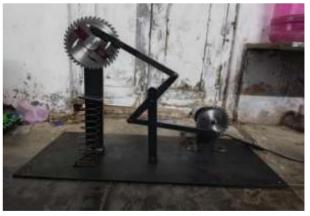
**b. Reciprocating Action** A mechanism, which includes a crankshaft and beam engine, transforms the motor's rotary motion into reciprocating motion. This mechanism causes the blade to reciprocate along the work piece. This reciprocating hacksaw
