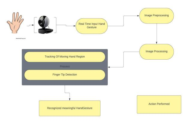
Hand Gesture (Input): Represents specific hand gestures recognized by the system for controlling the cursor.
