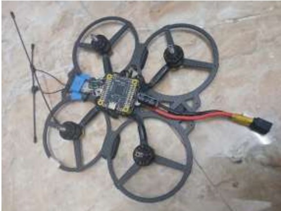
Fig. 5: Final Coated Drone Assembly Prior to Submersion Testing
