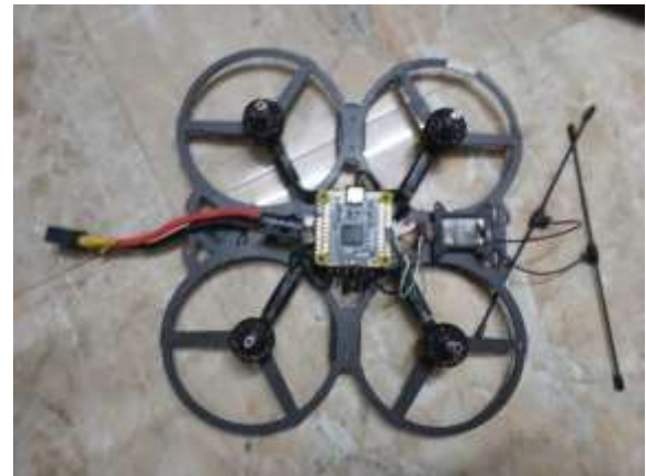
Fig. 1: 145 mm Carbon Fibre Structural Frame with Central Avionics Stack
