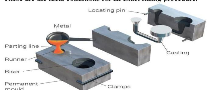
Figure 1.1: Gravity casting process
