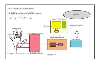
A simple robotic parallel manipulator is implemented employing embedded systems integrated with set of sensors more than one type of sensor is implemented together to control input data from the human limb. Initially, a data set is collected on map to equivalent certain actuations at the manipulator and then using an appropriate machine learning algorithm to control data values for continuous position of actuator generation.
