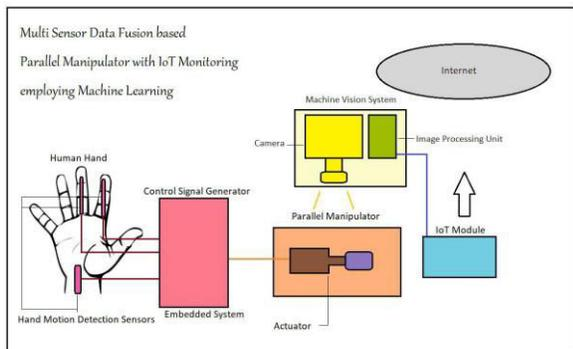
A simple robotic parallel manipulator is implemented employing embedded systems integrated with set of sensors more than one type of sensor is implemented together to control input data from the human limb. Initially, a data set is collected on map to certain equivalent actuations at the manipulator and then using an appropriate machine learning algorithm to control data values for continuous position of actuator generation.
