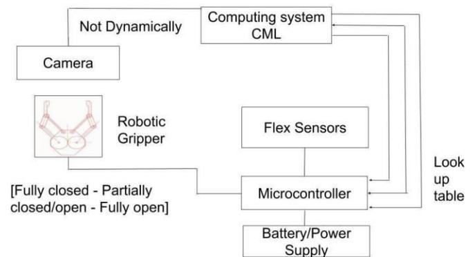
Hardware implementation of the parallel manipulation is carried out by collecting the flex sensor signals from glove which is attached to hand trained AI, capable of choosing better signal from flex. A control signal is generated simultaneously to run the
