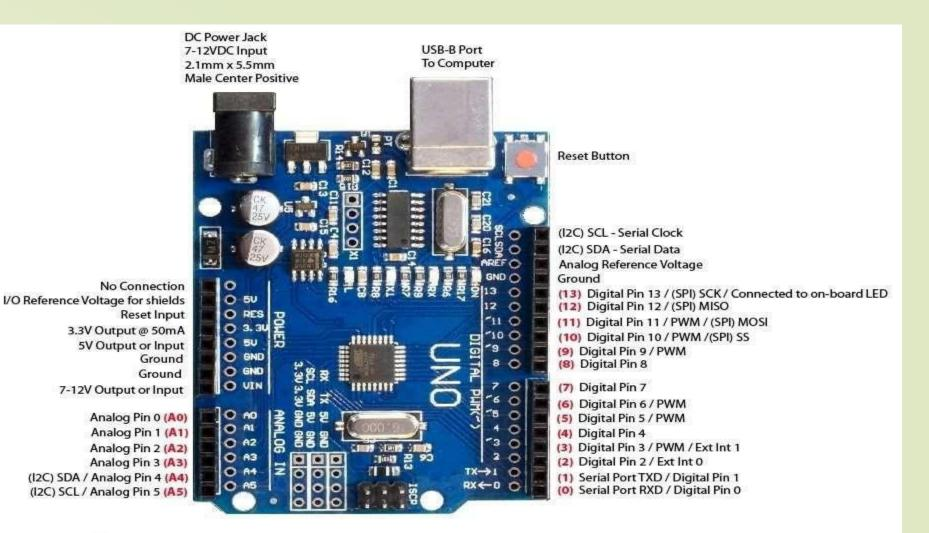
**Red** numbers in paranthesis are the name to use when referencing that pin. Analog pins are references as A0 thru A5 even when using as digital I/O
