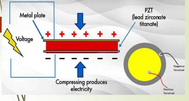
Squeeze certain crystals (such as quartz) and you can make electricity flow through them. The reverse is usually true as well: if you pass electricity through the same crystals, they "squeeze themselves" by vibrating back and forth. That's pretty much piezoelectricity in a nutshell but, for the sake of science, let's have a formal definition:
