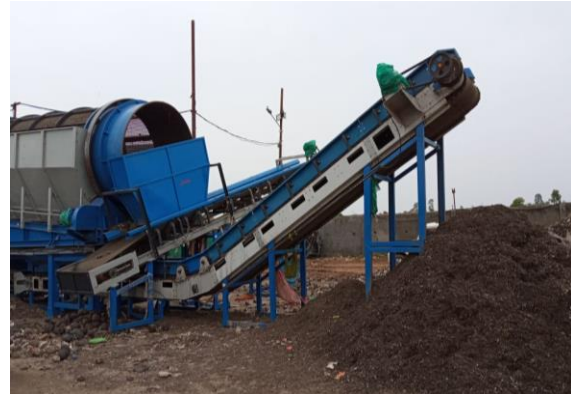
(g) Bio-mining Facility for legacy waste treatment
