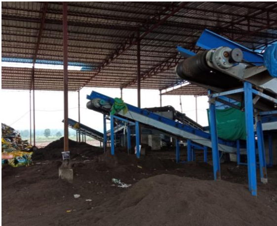
\ (b) RDF Processing unit:
