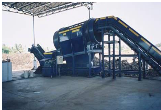
Fig -2: PRE-SEGREGATION MACHINE
