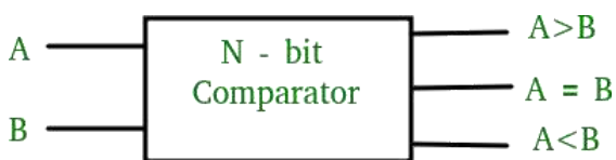
Fig-3: Block Diagram of Comparator
