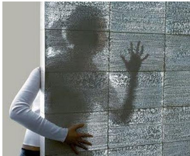
Fig. 5: Transparent concrete wall
