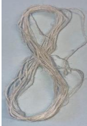
Figure 3: Banana -Cotton yarn (60B:40C)
