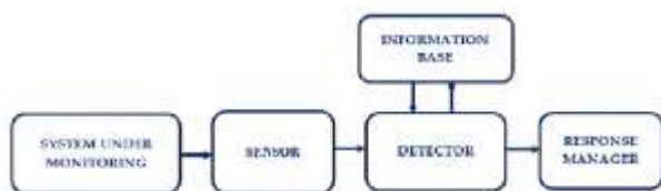
Fig -2: General block diagram of an intrusion detection system.
