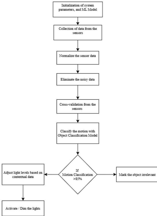
Fig. 4.1: A simple flowchart depicting the work-flow of the algorithm used.
