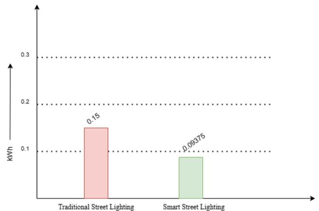
Fig. 5.2: Comparison of operation cost of traditional street light vs smart street lighting systems
