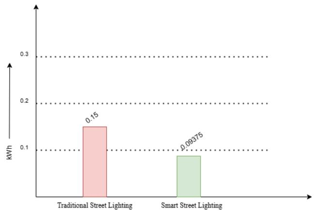
Fig. 5.1: Comparison of Energy consumption of traditional street light vs smart street lighting systems
