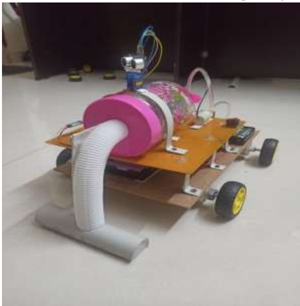
Figure 4: DuoClean Prototype: Fully assembled with ESP32, sensors, and cleaning modules.
