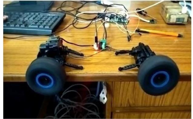
Fig.2 Test run of the robot without the chassis
